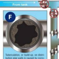
Tuberculation, or build-up, on distribution pipe walls is caused by corrosion and microbial activity. Excessive tuberculation affects both the quality and quantity of water supply. Distribution system deficiencies are responsible for over 25% of water-borne disease outbreaks in the United States each year.
